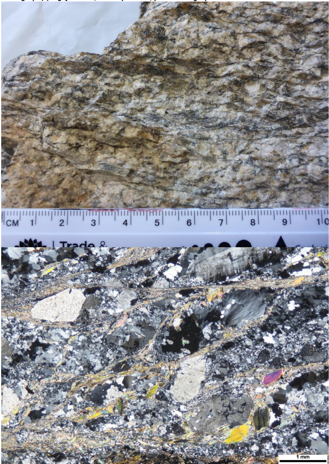
Figure 1 Photomicrograph in cross-polarised light of the mylonite showing well-developed S-planes (lower-left to top-right) and C-planes (left-to-right) wrapping around porphyroclasts of plagioclase (upper-left and below-centre), K-feldspar (above and to the right of centre) and muscovite (lower-right).
